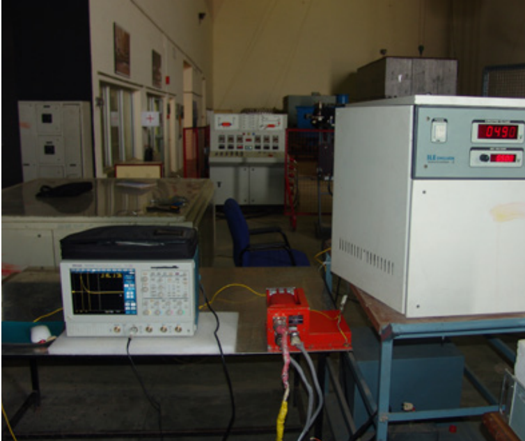
Indirect Lightning test on Aircraft equipment
