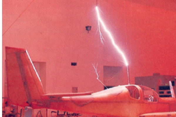
Lightning Attachment Test on Hansa Aircraft
