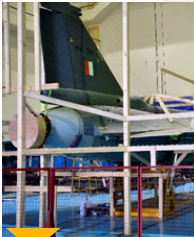
Light Combat Aircraft under going Lightning Test
