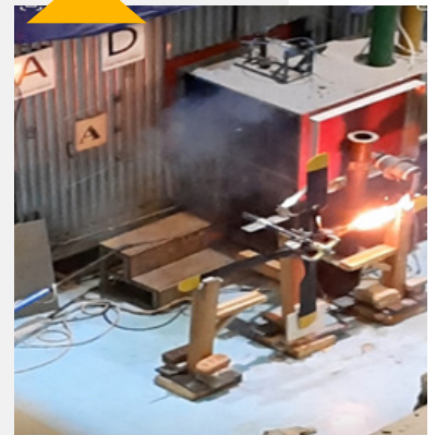
High Current Testing on a Helicopter Tail Rotor
