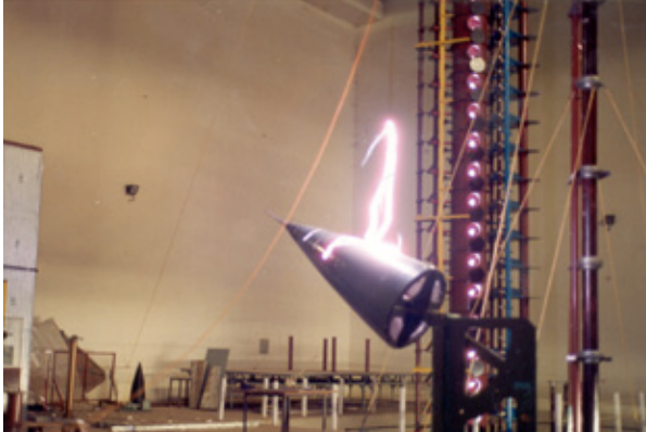
Lightning Attachment Test on Light Combat Aircraft Radome
