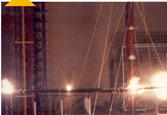
High Current Testing on a Helicopter Main Rotor Blade
