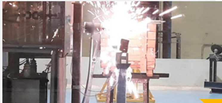
High Current Test on Spiral Antenna
