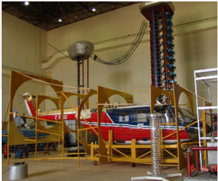
Indirect Lightning Effect Testing on a Helicopter
