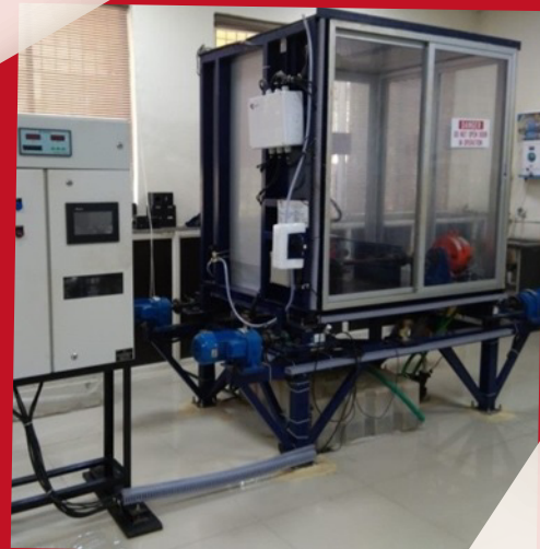
Vibsim I.I "Active Anti-vibration Mount System for Heavy Machineries payload"
