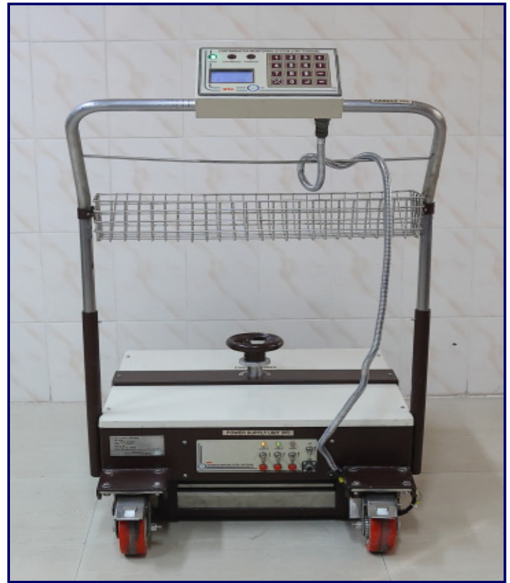
CONTAMINATION MONITORING SYSTEM – TERRAIN
