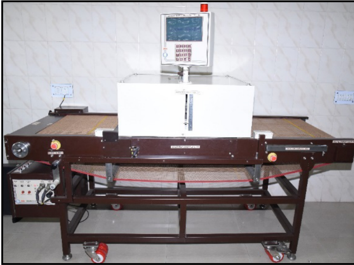
CONTAMINATION MONITORING SYSTEM – LINEN
