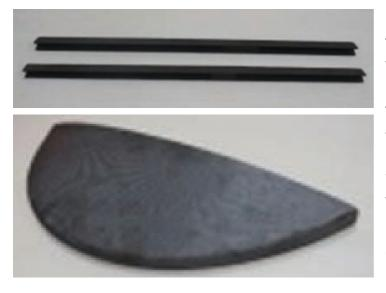
The components are made by Chemical Vapour Infiltration and Deposition (CVI-CVD) of SiC into Carbon fibre performs. The Cf-SiC composite has excellent thermal shock resistance and strength retention up to 1500 °C. The Nose Tips & Wing Leading Edges of Hypersonic Vehicles have been developed to resist high heat flux and temperatures. These are potential thermo-structural material.
