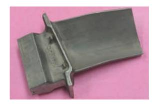
The castings are produced via vacuum investment casting process using Ni-base superalloys. Ceramic silica cores are used to get hollow cast components. Single crystal turbine blades and twin vanes are produced by using orthogonal grain selector from advanced Ni-base single crystal alloy. These components have been developed for gas turbine engines of aircraft for high efficiency, high thrust and low specific fuel consumption.
