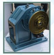
HISPEL is a high speed gearbox designed and developed to transmit 25kW power and to step up the output from commercially available electric motor to 1,10,000 rpm. Speed from the input motor is stepped up in three stages and is designed with combined straight and epicyclic gear trains. This gearbox is intended to provide the drive to test the performance of units/ accessories fitted of small turbofan class engines. Gearboxes have been manufactured, assembled and tested to 1,10,000 rpm
