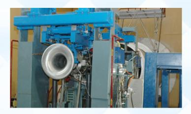
STFE is a Twin spool, low By-Pass Turbo Fan, Aero Gas Turbine Engine intended for use in unmanned air vehicle. The engine is controlled by Digital Engine Control Unit (DECU). STFE engines are being manufactured and integrated by Indian industry partners. Experimental trials are in progress. It will be inducted into services after the certification
