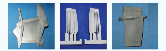
Indigenous single crystal Blades and Vanes are designed and developed for High Pressure Turbine rotor blades and nozzle vanes. This critical Hot end technology is developed for life enhancement to meet engine life requirement. High Pressure Turbine Rotor (HPTR) Blade casting is completed and certification is under progress. High Pressure Turbine Vane casting and inspection is under progress.
