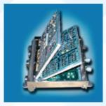
Design and Development of fully qualified electronic control units along with necessary system software, application software and control laws. It is built around dual redundant architecture to meet mission reliability. The AFADEC is designed, developed, qualified and successfully integrated & tested in Kaveri Derivative Engine.
